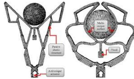
Fig. 2. Example of compliant underactuated gripper
