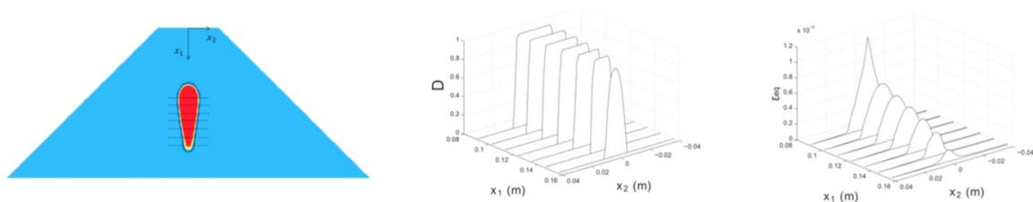
Figure: Notched trapezoidal beam: damage and equivalent strains around the crack. Evolution of the localization zone
