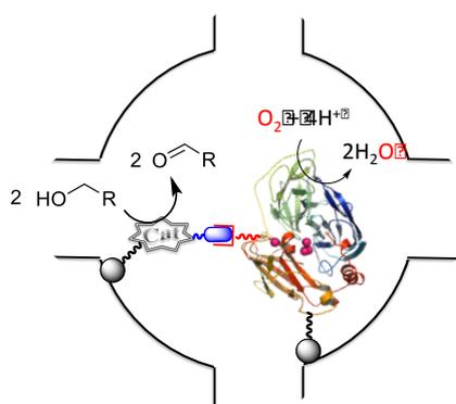
Schematic representation of a porous silica foam immobilized hybrid catalyst for alcohol oxidation.
