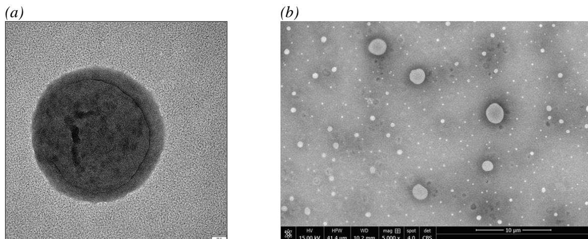
*Figure 1 : TEM (a) and SEM (b) images of magnetic microbubbles*
