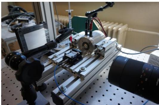
In the last few years, a home-made apparatus has been developed in the laboratory. (fig. on the left). It allows following the motion of a water droplet (2-3 $\mu$ L) deposited on a textured surface vibrating horizontally between 10Hz and 200Hz. With this set-up we follow the droplet motion and displacement thanks to a fast camera (up to 3200 fps in full frame) and we get the droplet profile through image analysis.
