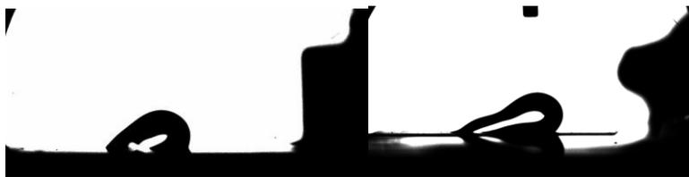
Fig. 2: Droplet on a smooth (left) and textured (right) surface vibrating at 47 Hz; amplitude is  $\sim 1$  mm
