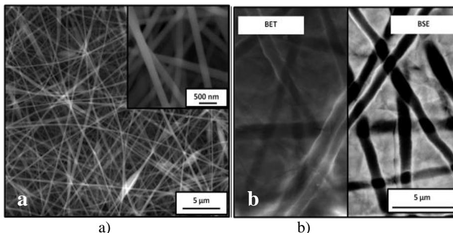
*Fig.1: a) : carbon base nanofibers network. b) CMC composite with carbon based fibers fillers.*
