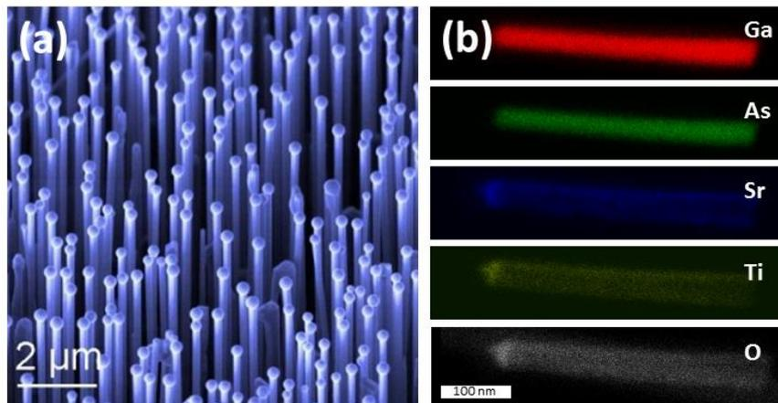
*Figure 1: Scanning Electron Microscopy image of GaAs nanowires grown using Vapor Liquid Solid method by Molecular Beam Epitaxy (a). Two-dimensional element mapping for a single GaAs / SrTiO<sub>3</sub> nanowire (b) [5].*
