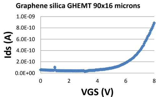
*Current-voltage curves for a  $90 \mu\text{m}$  (width) and  $16 \mu\text{m}$  (length) Graphene FET.*
